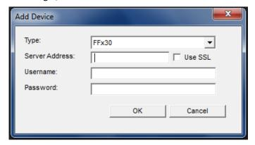
If the **Auto Discover Devices** feature was used, you may Right-click and select **Add** or double Left-click on the IP address or name of the FF240-IP unit that was detected. Use the 'X' in the upper right hand corner to close the Auto Discover window after you have added it to the client.
